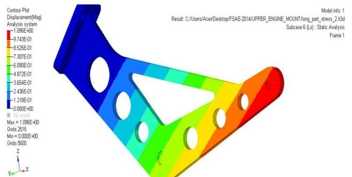
Fig.26. Displacement plot
