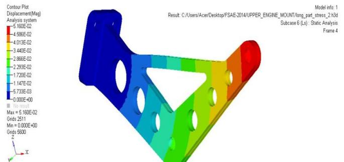
Fig.24. Optimized displacement plot
