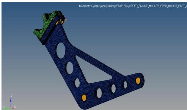
Fig.22. New meshed model
