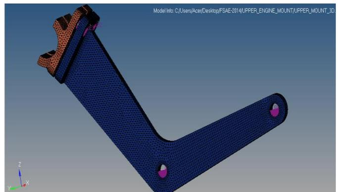
Fig.4. Meshed Assembly
