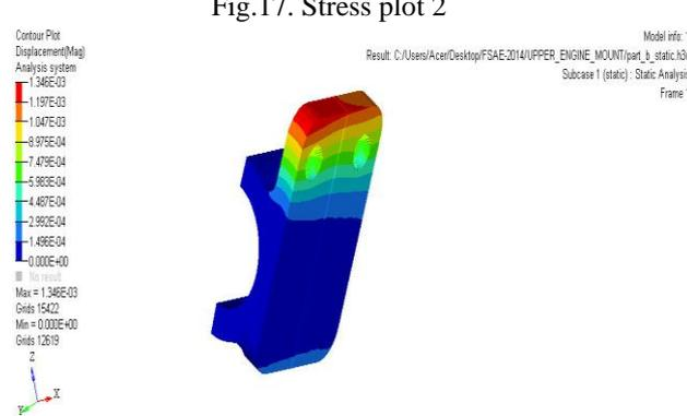
Fig.18. Displacement plot
