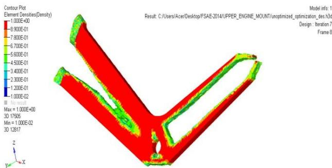
Fig.20. Optimization with removed material
