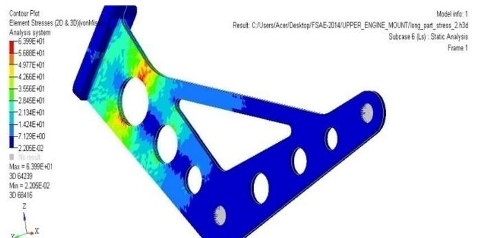
Fig.25. Optimized stress-plot for cornering and braking condition
