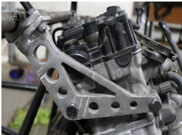
Fig.29. Installed Mount Bracket
